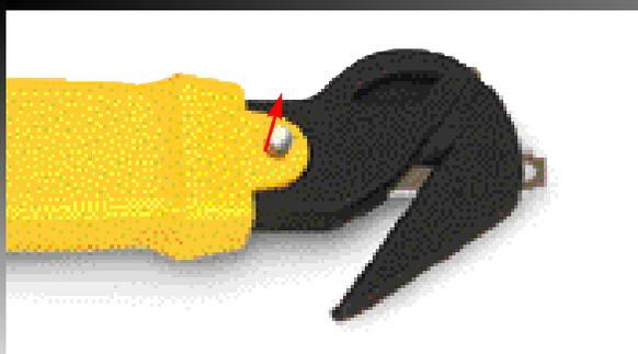
Push the tail of the locking pin through the back of the cutter. Therefore, you may need to push the tail of the pin against a hard object such as a desk or bench. The head of the pin will now be freed up enough to pull it upward until it has reached the top of its travel and clicks into place. The pin will then be clear of the blade hole. (The pin does not need to be removed from the cutter to effectively change the blade.)
